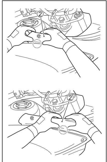
10. The fuel tank cover has fasteners behind the cover at the rectangle mark places.
